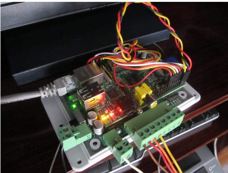
I tested the Opensprinkler Pi zener at 4.96V with the Toro power adapter. Didn't see any notes about polarity but I was hesitant about blowing something up on the first switch on.
