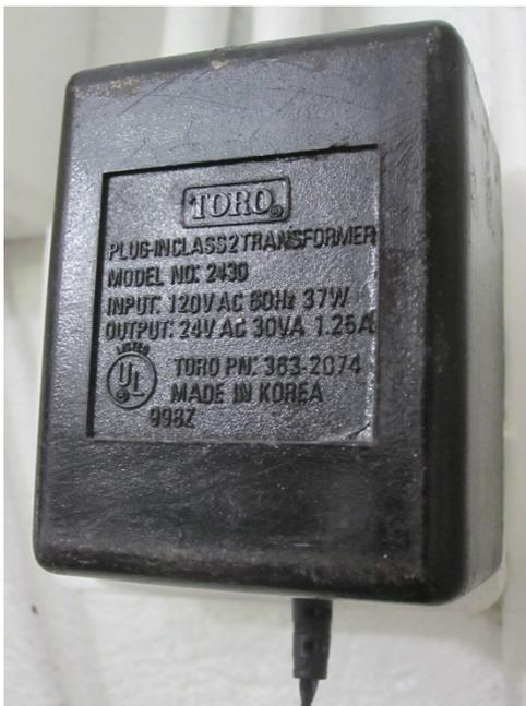
What luck! The power adapter on the Toro is 24V, exactly what we need for the Pi setup.
